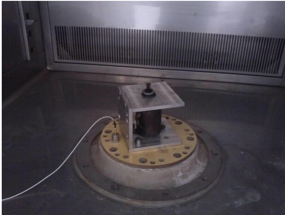
Figure 2 the motor is fixed on the vibration table with vertical direction
